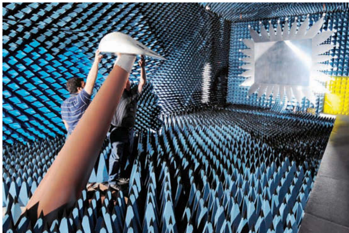
Researchers adjust a target for testing in GTRI's new compact range (courtesy Gary Meek, Georgia Institute of Technology).
